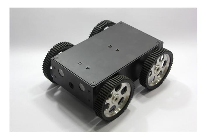
The DuctBot goes inside centrally air conditioned ducts-inspects and cleans it off dust and other impurities. It sends back real time video while inside the duct. It has powerful LEDs mounted which illuminate the dark duct. It comes with a simple joystick and a hand held monitor with which the operator can track and control the motion of the robot inside the duct.
