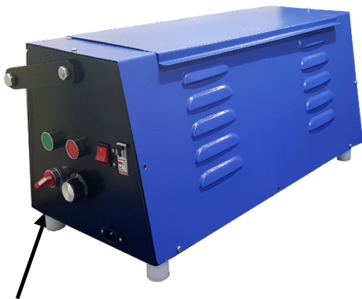
ON/OFF control with speed & direction change option
